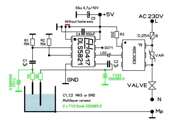
When operating water tanks with radiators, use safety devices marked in green. Factory default switching thresholds for detectors are set for electrodes up to about 8 cm. If you need a different sensitivity then you should set it like this:
