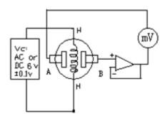
Sensor testing circuit pic. The resistance in this testing circuit should be greater than 100 G $\Omega$ , otherwise it would affect the sensor performance.
