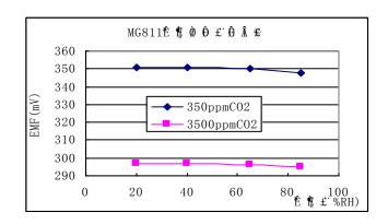
Fig6. Typical humidity characteristics
