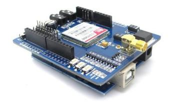
IComsat is a GSM/GPRS shield for Arduino and based on the SIM900 Quad-band GSM/GPRS module. It is controlled via AT commands (GSM 07.07,07.05 and SIMCOM enhanced AT Commands), and fully compatible with Arduino / Iteaduino and Mega.
